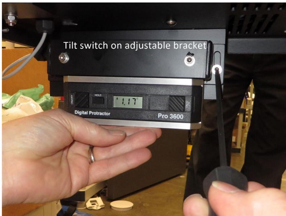
The bracket can then be rotated around the left hand screw through an angular range permitted by the slot on the right hand side.
