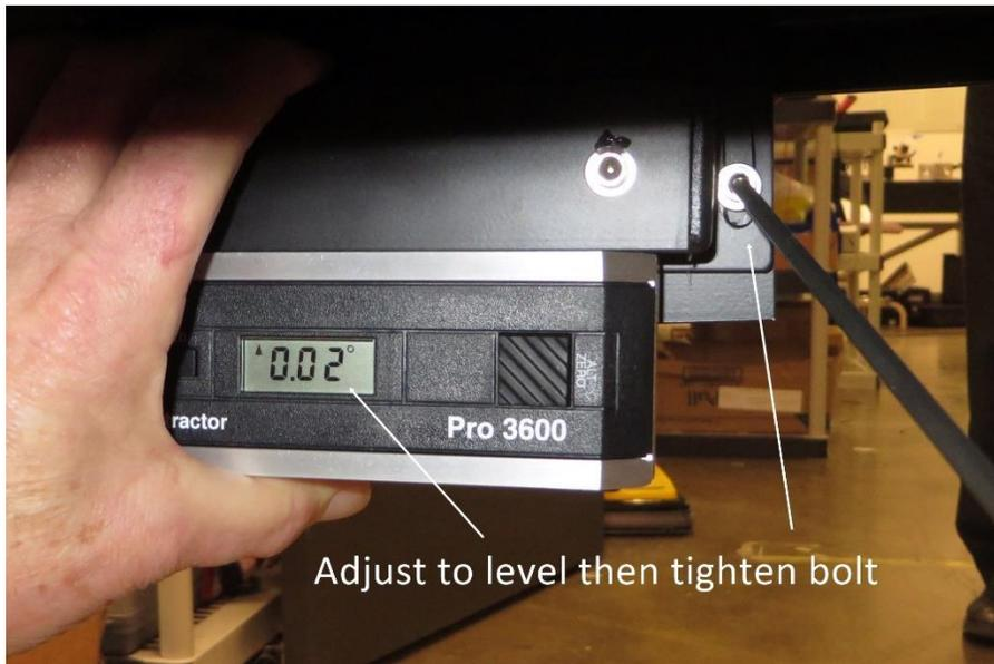
The “closed” range of the tilt switch is within the angular range of +0.5 degrees and -0.25 degrees. A small deviation within this range will not affect functionality.
